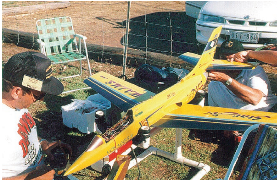
Chris Mounkley built this Star Jet which is powered by a JPX-260 turbine. Note the maze of wiring in cockpit.
