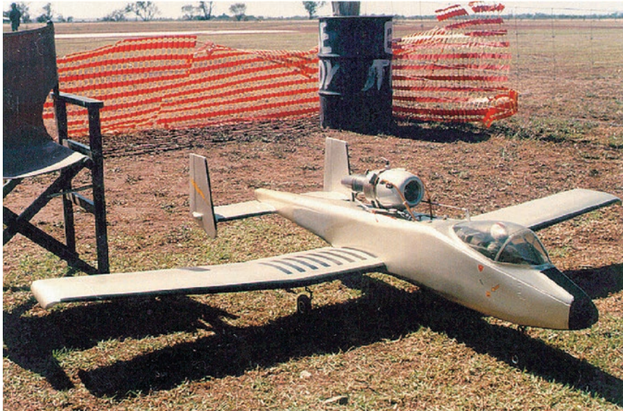
Kevin Dodds of Tingalpa, Qld built this semi-scale A-10 "wart hog". Powered by a JPX-T-240 turbine, the model weighs 7kg empty and 8.5kg fuelled. Maximum engine speed is 122,000 rpm!
