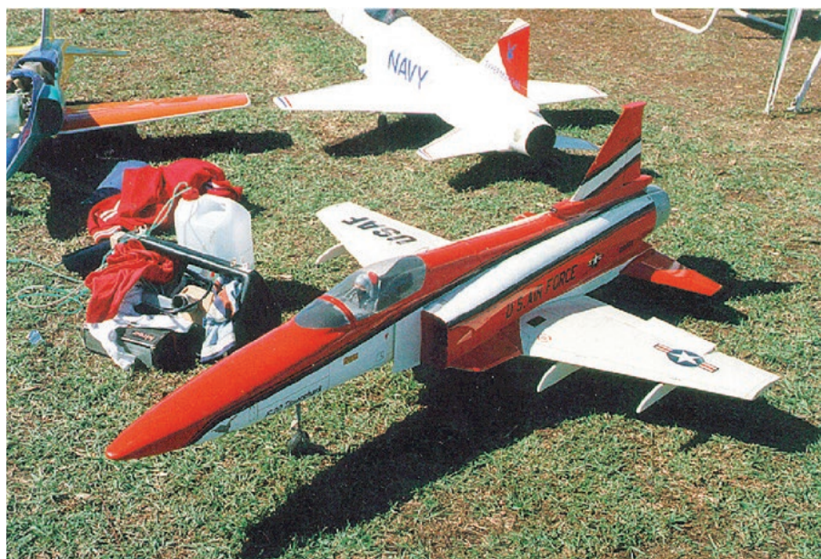
This beautifully finished model of an F-20 Tigershark was built by Brett Davies. It is powered by an OS91 engine fitted with a Ramtec fan. It is 1.82 metres long and weighs just on 6kg.
