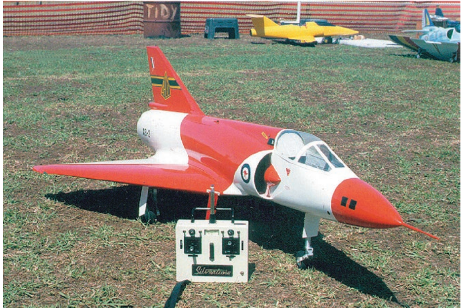
This Mirage was built from a Jet Hobbies Hanger kit. It is powered by a Golden West Models FD-3/67LS turbine and controlled by a Silverstone transmitter. It has a wing span of 1.09m, length of 1.56m and a weight of 5kg. It carries 1.75kg of kerosene.
